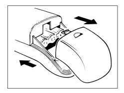
**NOTE:** This product operates optimally with either a 2.4V, 300 mAh, NiCad battery (supplied) or a 3.6V, 270 mAh NiCad battery (part number 213-013-9-001).
